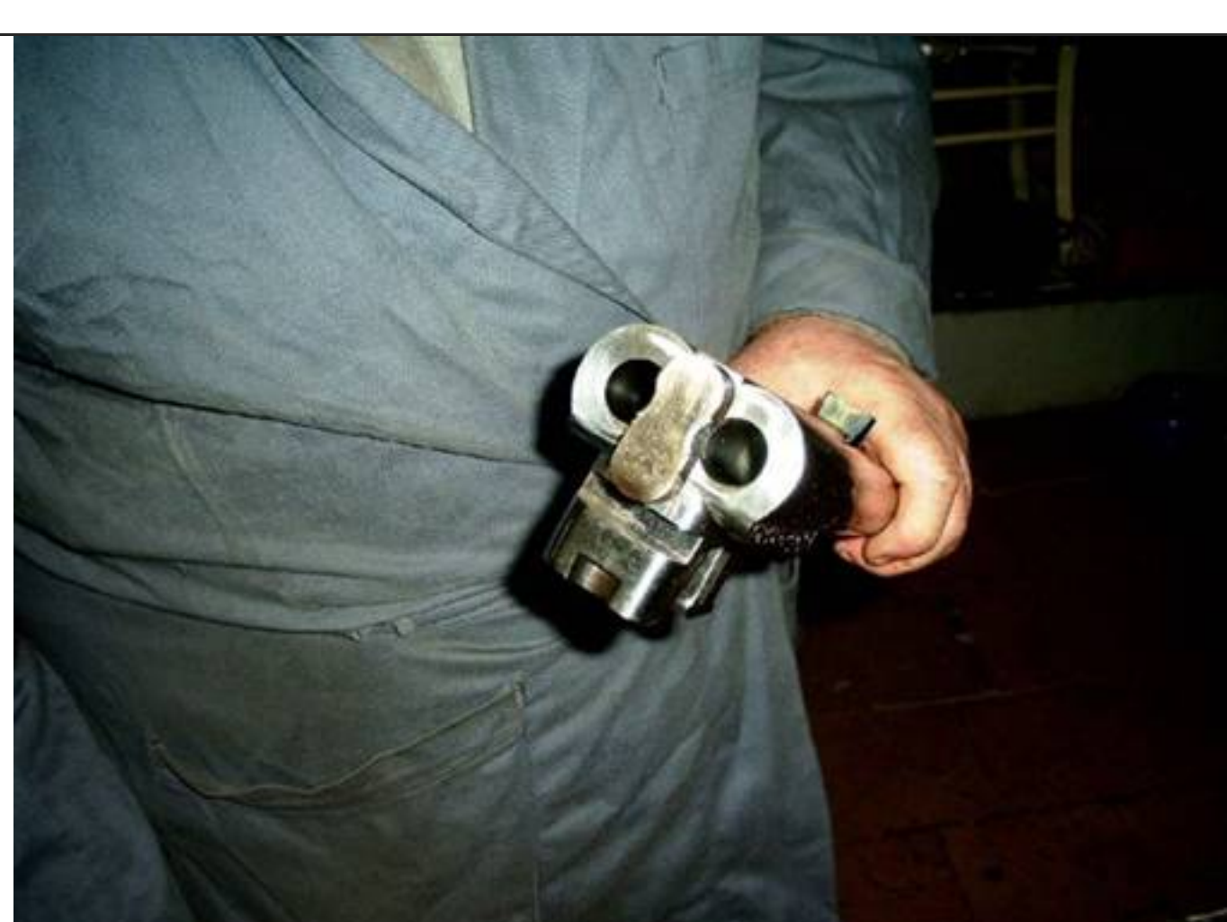
Massive Integral Underlugs and Extractor on 577 Tyrannosaur.
