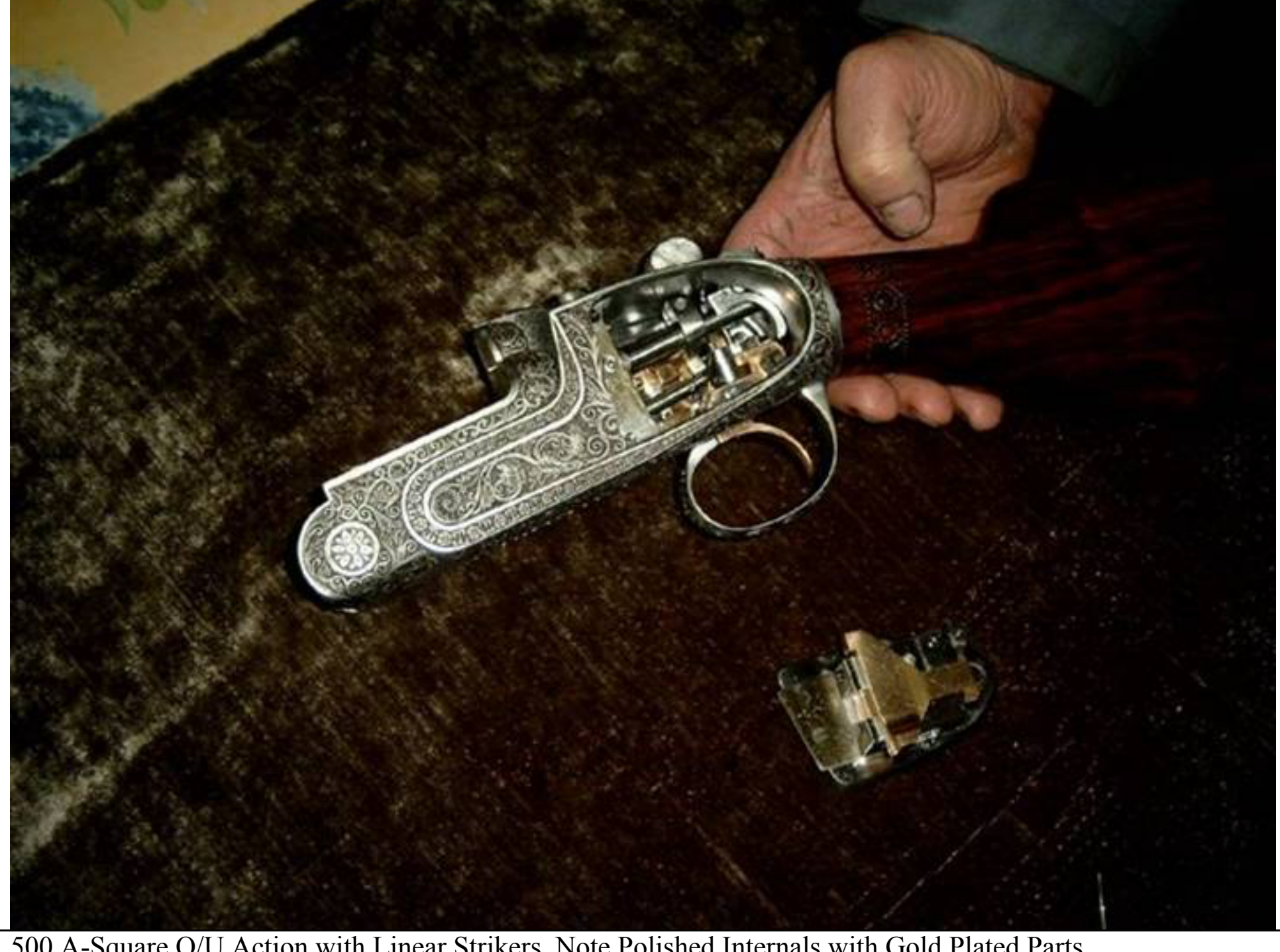
500 A-Square O/U Action with Linear Strikers. Note Polished Internals with Gold Plated Parts
