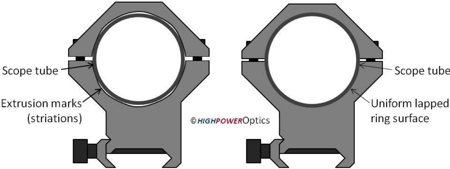
Figure 2. Left: Non-uniform contact between ring and scope tube due to extrusion marks (striations). Right: Uniform surface contact between ring and scope tube after lapping the rings.
