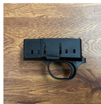
**R8 Blaser Fire Control Assembly, Trigger**
