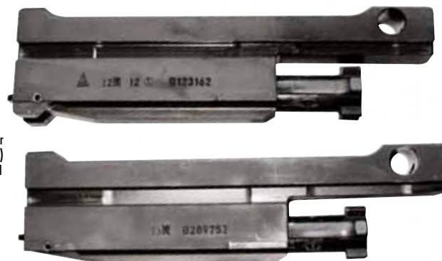
Comparing breech block carrier of the CZ 805 BREN A1/A2 (top) and CZ 805 BREN S1
