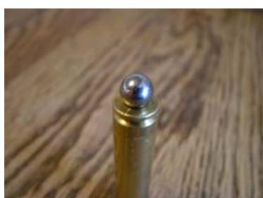
You must support the web of the cartridge from inside. If you have a very rigid work bench you could drive the ball with a hammer, or you could use an arbor press or a hydraulic press. I decided just to give a vise a try. It did not move quite enough metal so I put a c-clamp over the outside and that gave me enough pressure. I didn't photograph using the C-clamp.
