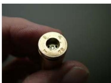
Then a .076 drill was run all the way through and deburred on both sides.
