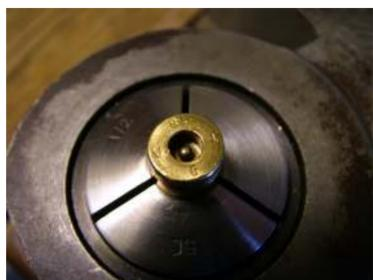
You can't easily drill this anvil out as the drill will run off and damage the wall. You could locate the fixture under the spindle and plunge an end mill to cut it. I simply made a .214" dia. cutter from a gage pin that would cut on the end only. Easy to do with a Dremal tool. Two negative rake (for brass) cutting edges just like a drill and relieved behind the cutting edge. The smooth outside wall will not cut and the edge being flat doesn't push off center.
