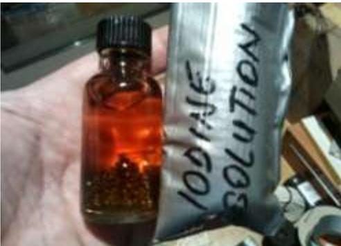
Iodine saturated solution with its neoprene-duct tape makeshift pouch (to keep it warm) and identification (note the iodine crystals at the bottom, about 4-8 grams). **NOT SUITABLE FOR PREGNANT WOMEN OR FOR INDIVIDUALS WITH THYROID DYSFUNCTIONS.**
