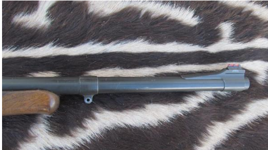
Figure 6 - Front of rifle showing barrel band sling swivel and front sight.
