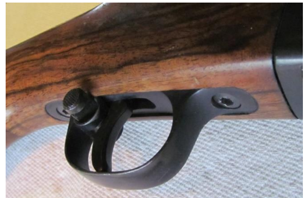
Figure 5 - Custom "Cross Bolt" Safety. Safety in "ON" position in this photo.
