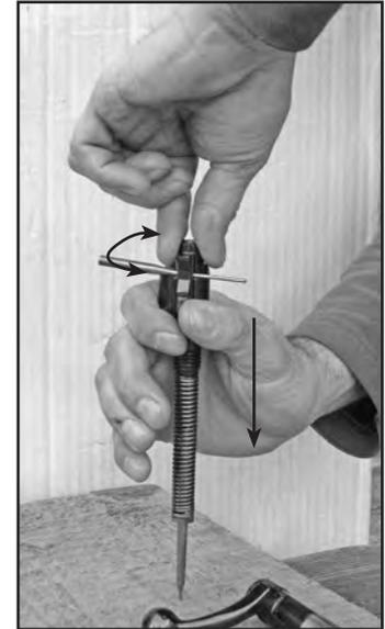
Fig. 15> Stripping of hammer mechanism
