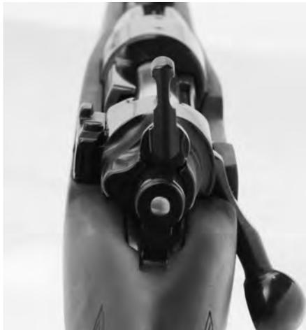
Fig. 11> Position of thumb-lock safety in stripping of model M98
