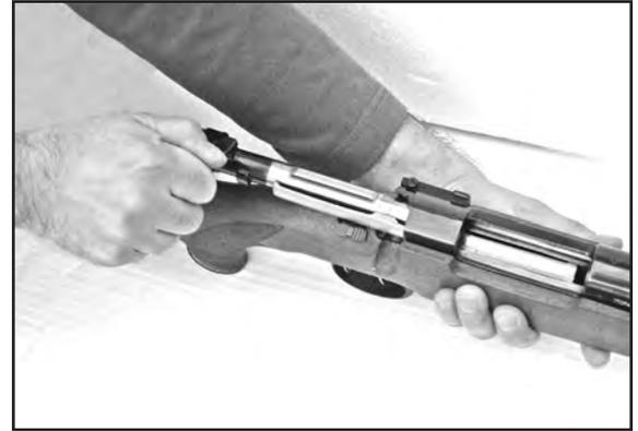
Fig. 6> Bolt in rear position
