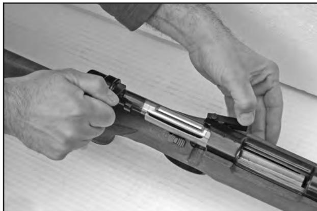
Fig. 12> Separation of bolt assembly from the sporting rifle
