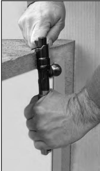
Fig. 13> Compression of hammer spring
