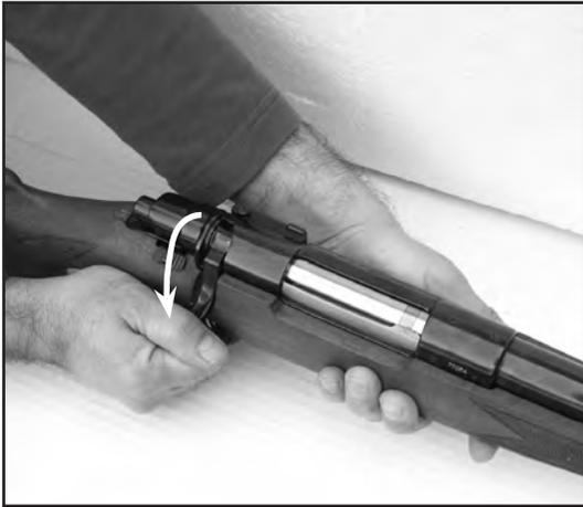
Fig. 8> Bolt in locked position
