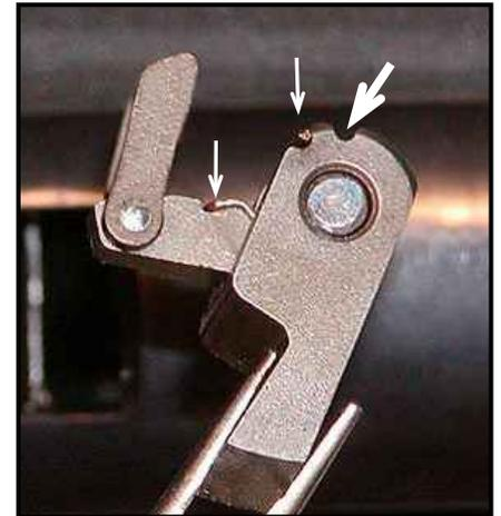
This view shows the frame upside down looking into the triggerguard slot. Insert the unsplined end of a 3/16 pin into the topmost hole in the LEFT side of the frame.
