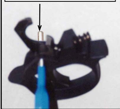
When the slave pin is in place, put a dab of grease on the ends of the barrel catch and trigger return springs and insert those ends into the holes they reside in, and they are less likely to fall out when hands are at a premium.
