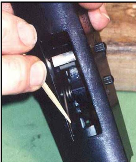
With the triggerguard assembled, you ready to add a dab of action grease onto any area(s) like the sear tip etc. that you may have rubbed the lube off of while doing this reassembly.
