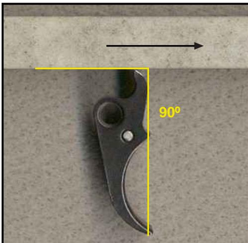
The photo at right shows how to hold the trigger and stone correctly, not the exact angle to stone...
