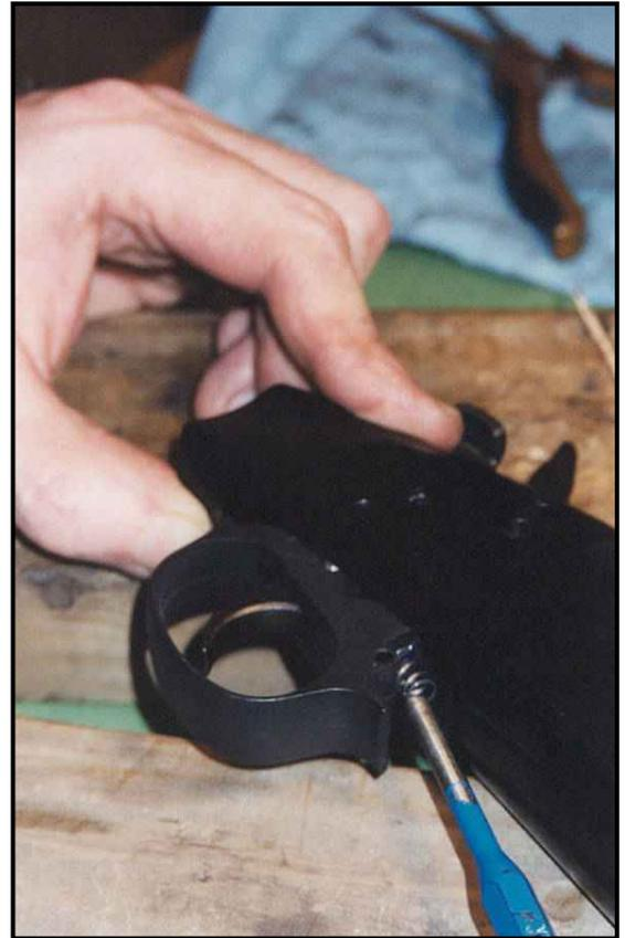
Have the large punch and the two triggerguard pins near your right hand to access easily. You **MUST** have the catch lever raised with your left finger to have (barely!) enough clearance for the barrel catch spring.
