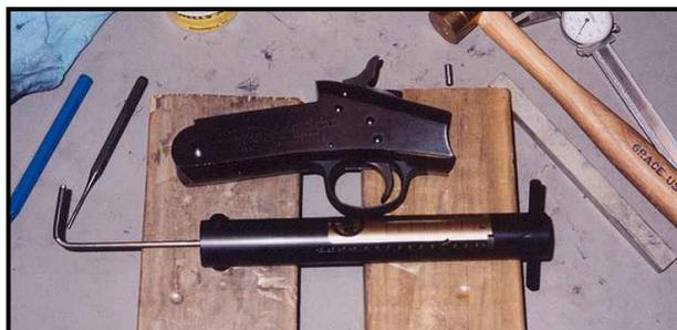
To do the final pin seating, reverse the wood (or metal) fixture to the left side of the frame and make a flopped version of the 2 x 4, frame and fixture clamped sandwich from the disassembly instructional. Pad that fixture if you made a metal one to avoid scratching the frame.
