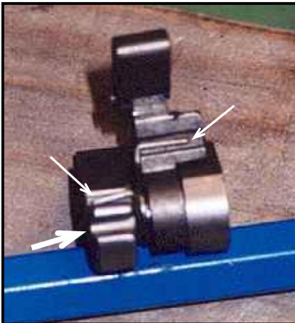
This is not easy to do, so be patient. In these two views of the catch/lifter assembly, note the thinner arrows pointing to where the "legs" of the lifter spring must sit in the two parts.
