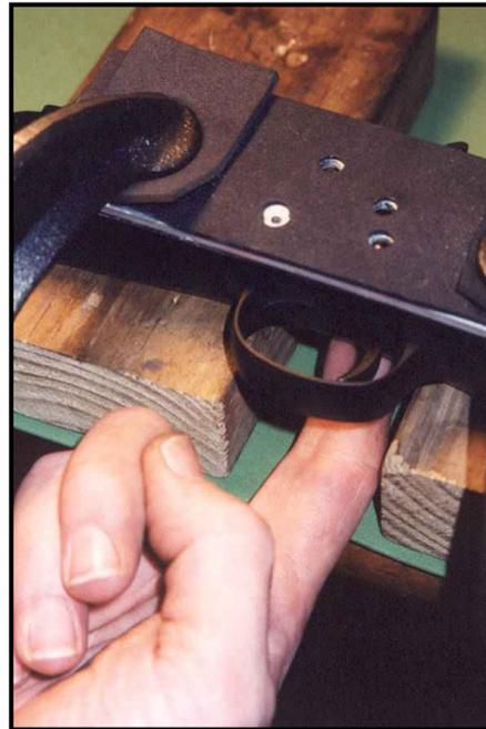
Remember to check safety function and pull weight once more after seating the pins fully - safety first! When you're satisfied with your work, reassemble stock and barrel in the reverse order of the disassembly instructional and enjoy your new trigger.
