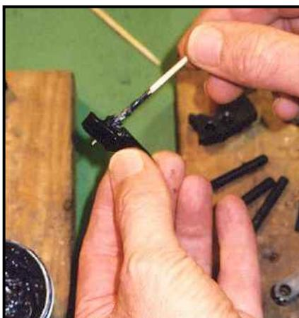
Use toothpicks to spread the lube inside holes and evenly across all surfaces that you polished. Set pieces aside after lubing on a piece of paper towel ready to be reassembled.
