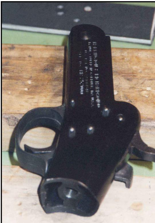
Test function before reseating the splined action pins fully. You don't want extra wear on the frame and pins by finding out after you seat them that something is wrong.
