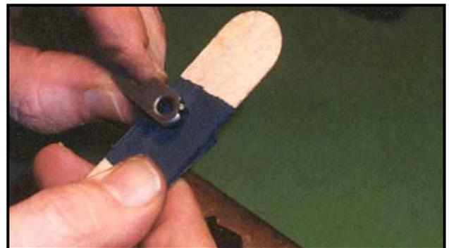
600 grit wet sandpaper wrapped around the 5/32 punch does nicely to polish the insides of holes on the hammer, trigger, lifter, extension and catch. Use a popsicle stick and sandpaper to smooth any rough spots in the slot inside the disassembled barrel catch. Remember that you are lightly smoothing, not enlarging the holes.
