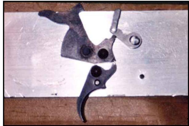
All pin holes, pins and bearing surfaces must be smoothed while taking care not to enlarge pin holes or reduce the pins they ride on by more than one or two thousandths of an inch. Any more than that and undesirable play and slop will creep into the trigger pull. The areas highlighted below in yellow will require polishing; the exact tools and methods best used will be shown in the pages that follow.
