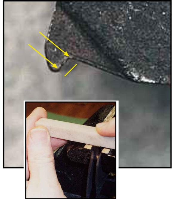
I would only stone the hammer hook as indicated above and give the sear about 10 to 20 light strokes at the 90° angle shown below, then reassemble and check pull weight. If still too heavy give the sear section about 20 more light strokes on your oiled stone. Make sure to keep the whole surface you are stoning in contact at the correct angle for the complete stroke to avoid rounding off the corners of the engagement surface. Light strokes means almost no downward pressure on the part at all.
