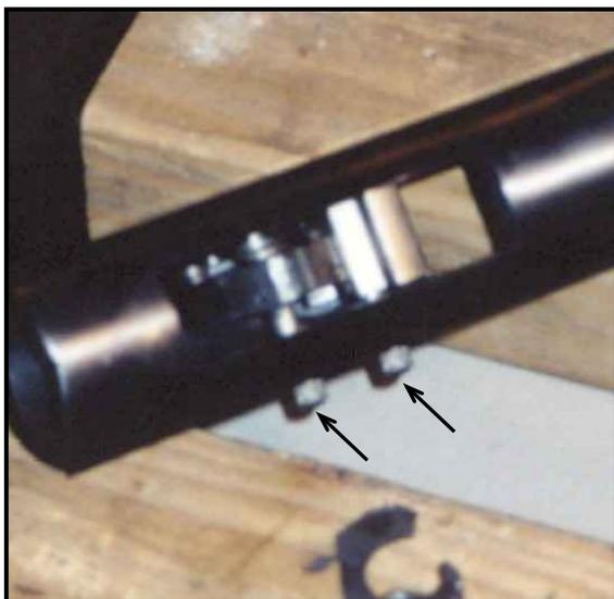
The two black arrows are pointing to the splined ends of the hammer and barrel catch pins barely touching the left frame side.
