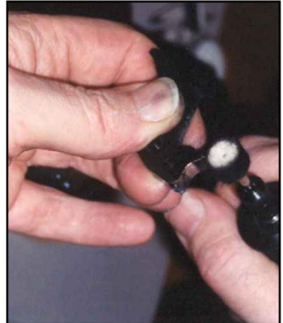
Note how rough this surface of the hammer is. The surface I'm pointing to only bears on the sear section of the trigger while cocking, but once you stone the sear smooth, why would you want it to rub over and over on a rough surface?
