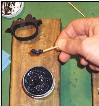
Use generous amounts of lube at this point, as the handling required to reassemble the action parts will tend to remove a good bit of what you apply.
