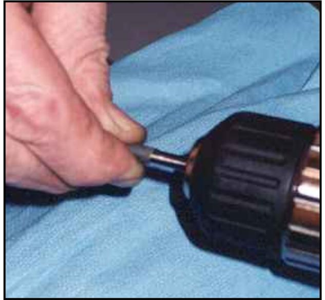
Gauge your pins with calipers before polishing. Even if they don't get as shiny as the one in the photo, stop when you have removed a max .002" of material.
