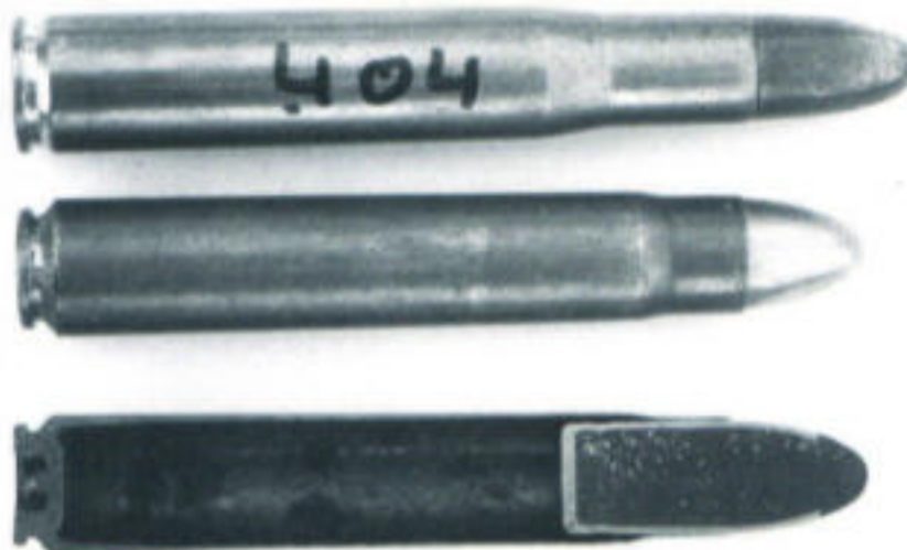
The sectioned 11.2 x 72 clearly shows how deep the bullet was seated, eliminating a considerable amount of powder space. If loaded to the same overall length like the .404 Jeffery, the 11.2 x 72 Schüler would deliver vastly superior ballistics.
