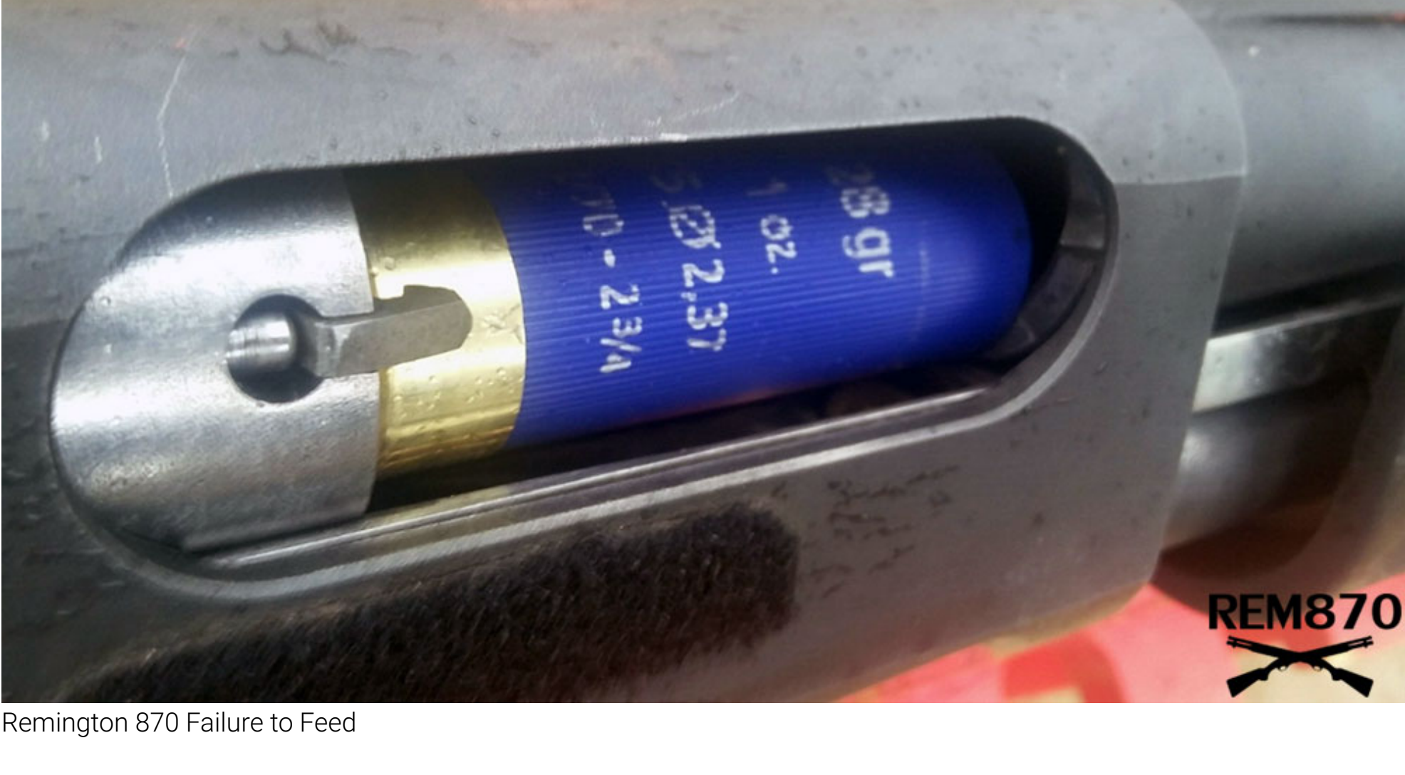
Remington 870 Failure to Feed
