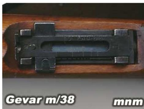
*Note the rear sight has the letter "T" stamped at the top of it. This denotes that the sight is calibrated for the m/91/41 139 grain bullet. Also the sight functions differently than a typical Swedish Mauser rear sight. The elevator bar is moved forward on the m/38 to increase elevation where on the typical m/96 the elevator bar moves from front to back to increase elevation.*
