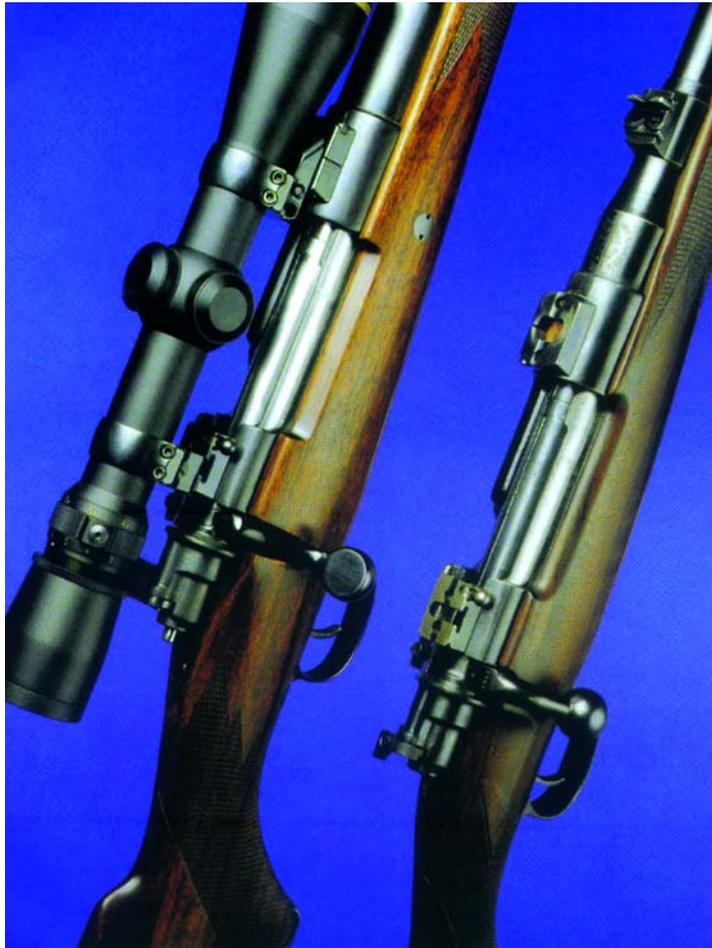
**Top: Cogswell & Harrison's innovative Certus rifle, one of the very few to survive, chambered for the .450/400 3/4in flanged Nitro Express cartridge. With its new and uncommon design and production principles, it was a forerunner of all modern machine-made firearms. Lower: Bolt-action rifles built on Mauser's Model 1898.**
