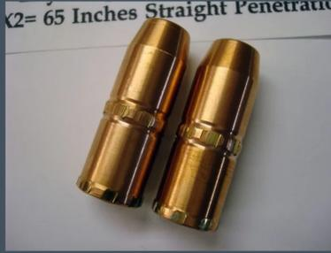
After such a successful barrel strain test with the 2 band bullet we decided that 4 bands would give the bullet more flexibility in seating depth, crimping, and neck tension. We had a 4 band design done by CEB and tested those successfully as well.
