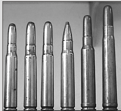
R - Old medium Bores. 8mm Mauser - the parent cartridge. 9mm Mauser, 9mm Mannlicher. The modern equivalents - .376 Steyr, .338 Winchester & .375 H & H.
