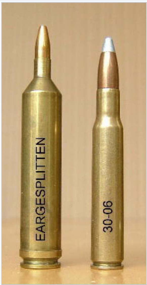
The .22 Eargesplitten Loudenboomer, designed by P.O. Ackley . Based on the .378 Weatherby Magnum , necked down to accept .224 caliber bullets. Next to a .30-06 Springfield for comparison.
