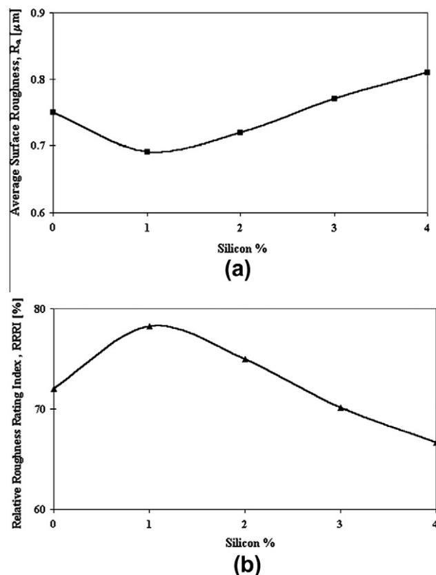
**Figure 12** Effect of Si content in cast Pb-free Si brass alloys up to 4 wt% on: (a) surface roughness “ $R_a$ ” and (b) relative machined surface roughness index “RRRI”.
