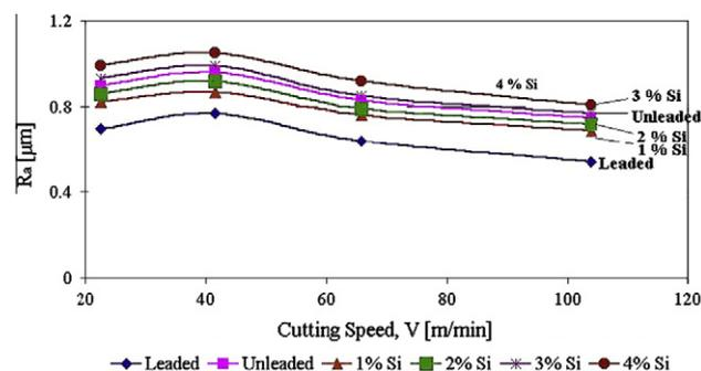
**Figure 11** Variation of average machined surface roughness “ $R_a$ ” of cast Pb-free Si brass alloys (Si up to 4 wt%) with cutting speed.
