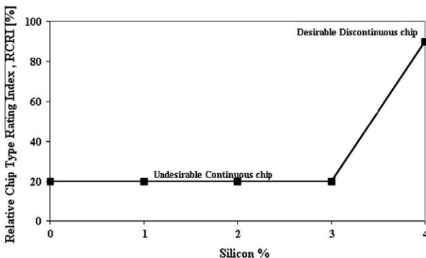
**Figure 13** Effect of Silicon Content on chip type.
