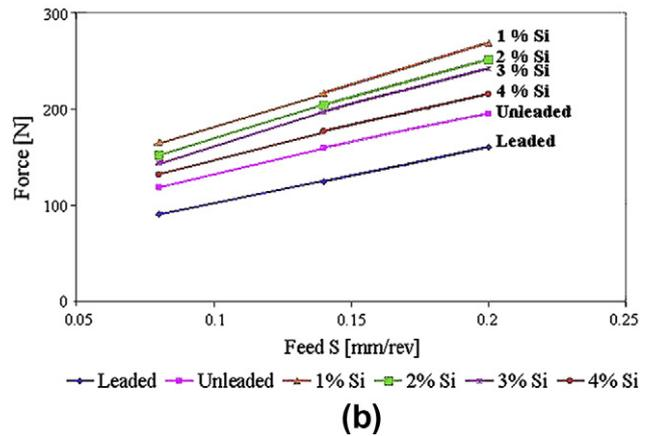
**Figure 5** Effect of cutting feed on the cutting force for the cast Pb-free Si brass alloys with different Si content up to 4 wt% (constant depth of cut of 0.5 mm and cutting speed of 104 m/min): (a) tool H123 and (b) tool H20.
