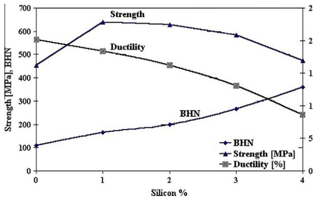
**Figure 3** Variation of mechanical properties of cast Pb-free Si brass alloys with Si content up to 4 wt%: ultimate tensile strength, ductility (elongation%) and hardness BHN).
