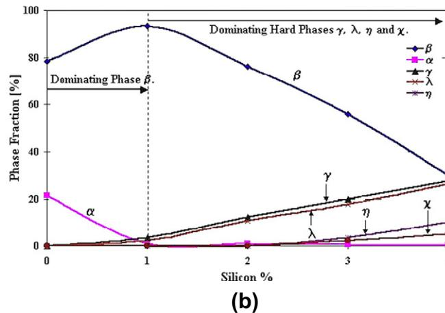
**Figure 2** Variation of the microstructure of cast Pb-free Si brass alloys with Si content up to 4 wt%: (a) micrographs indicating phases and their locations and (b) variation of phase's volume fraction with Si content.
