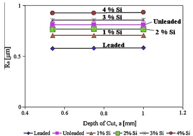
**Figure 9** Variation of average machined surface roughness “ $R_a$ ” of cast Pb-free Si brass alloys (Si up to 4 wt%) with depth of cut.
