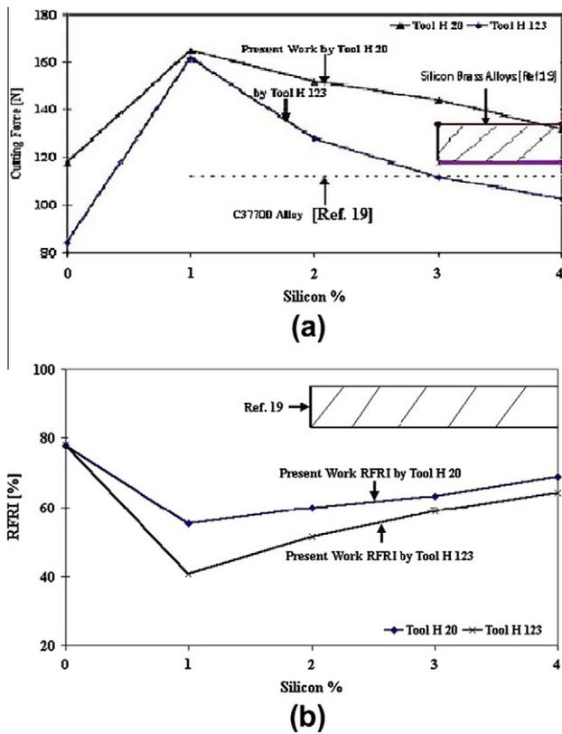
**Figure 7** Effect of Si content on: (a) cutting force and (b) relative force rating index “RFRRI”. The figure includes the present results on cast Pb-free Si brass alloys up to 4 wt% previous results on similar alloys after hot extrusion followed by heat treatment [19].
