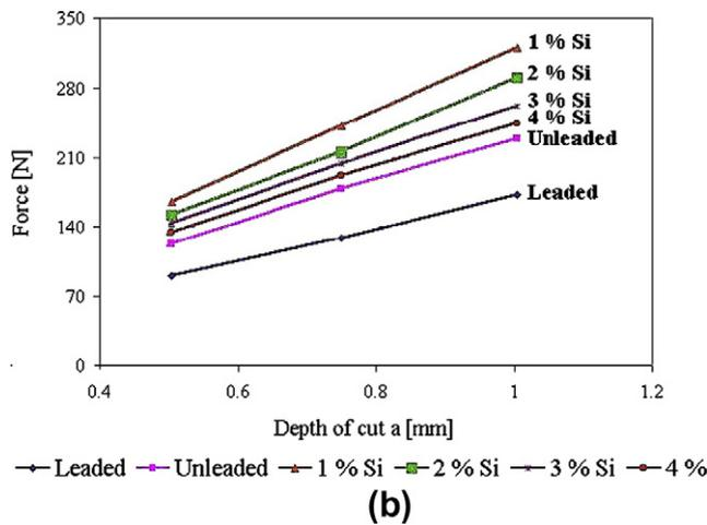
**Figure 4** Effect of depth of cut on cutting force for the cast Pb-free Si brass alloys with different Si content up to 4 wt% (constant feed of 0.08 mm/rev and speed of 104 m/min): (a) tool H123 and (b) tool H20.
