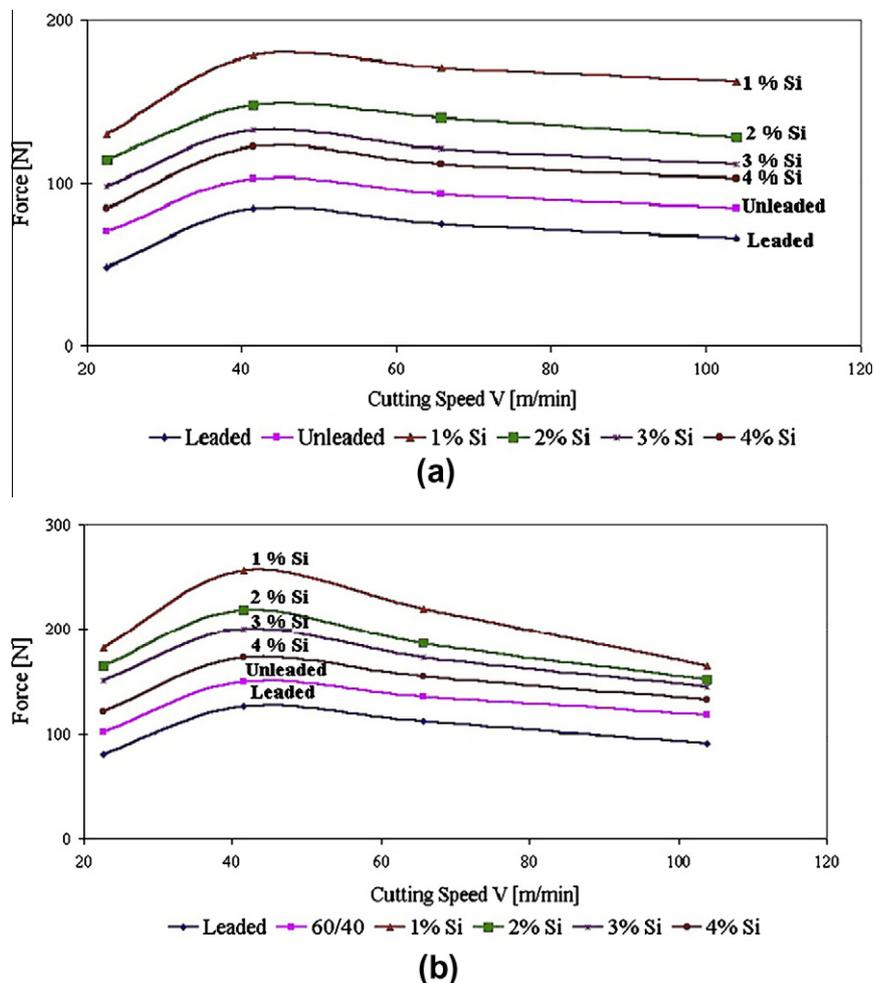
**Figure 6** Effect of cutting speed the cutting force for the cast Pb-free Si brass alloys with different Si content up to 4 wt% (constant depth of cut of 0.5 mm and feed of 0.08 mm/rev): (a) tool H123 and (b) tool H20.
