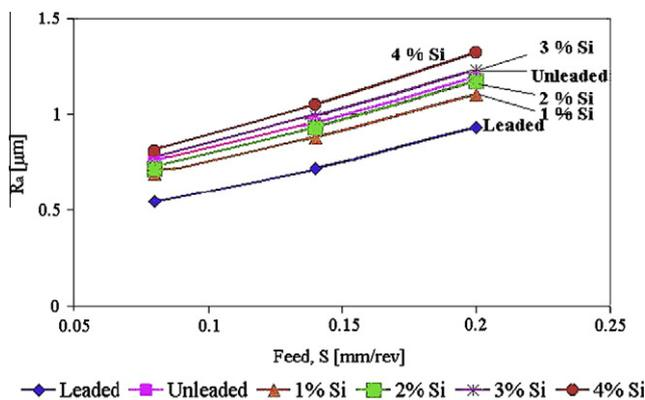
**Figure 10** Variation of average machined surface roughness “ $R_a$ ” of cast Pb-free Si brass alloys (Si up to 4 wt%) with feed of cut.
