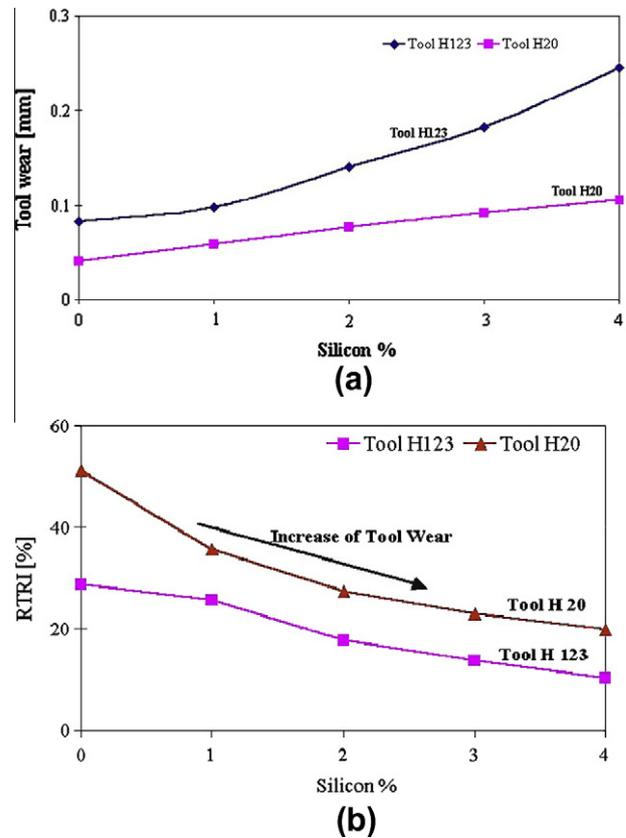
**Figure 8** Effect of Si content in cast Pb-free Si brass alloys up to 4 wt% on: (a) average tool wear and (b) relative tool wear rating index “RTRI”.
