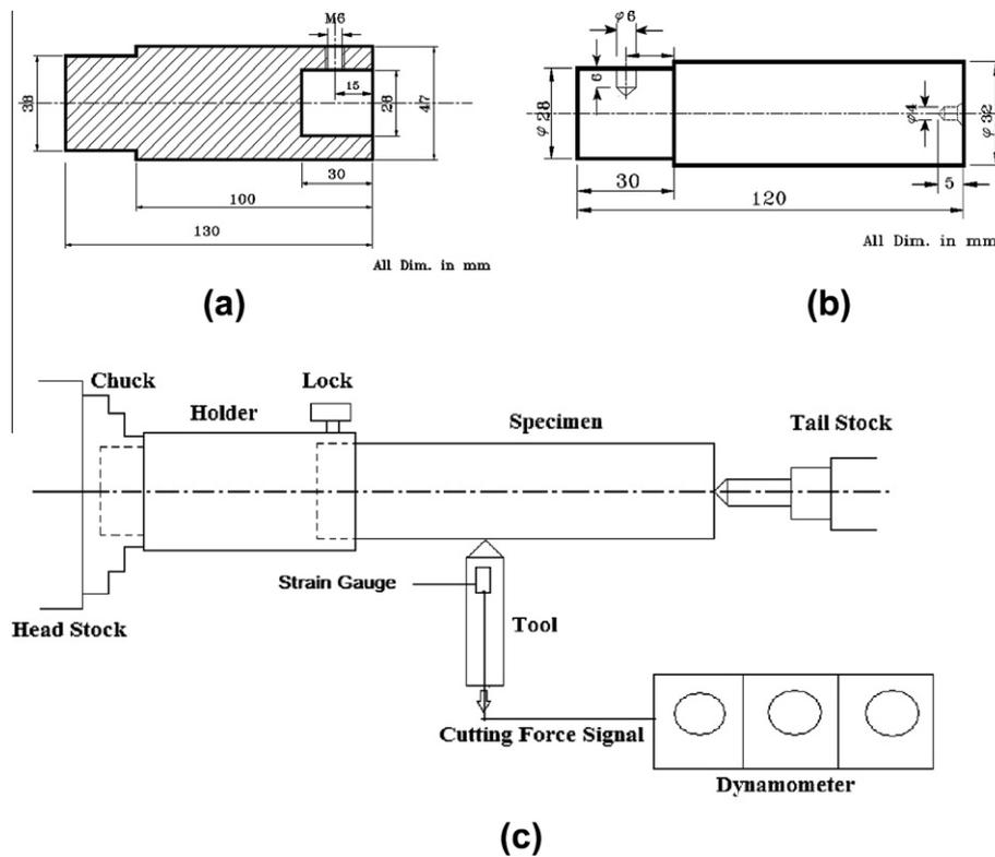
**Figure 1** Machinability test: (a) specimen holder, (b) specimen, and (c) sketch for the test arrangement.
