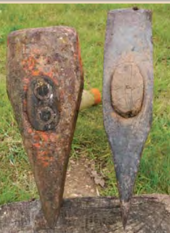
Above: Two classic splitting mauls – one with a very obtuse edge profile (left) and the other with a far more effective concave grind for maximum penetration.
