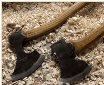
Above; two fantastic carving axes with asymmetric grinds, on the left a replica Viking axe made by Stefan Ronnqvist and on the right the Gransfors Carving Axe
